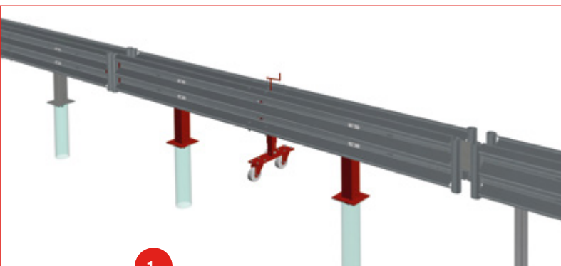
1. Lock the lifting device and rise the system
